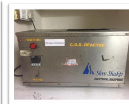
C O D Reactor
